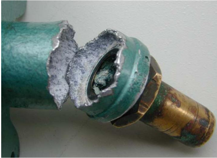
Corrosion of Al coupled with brass in seawater
