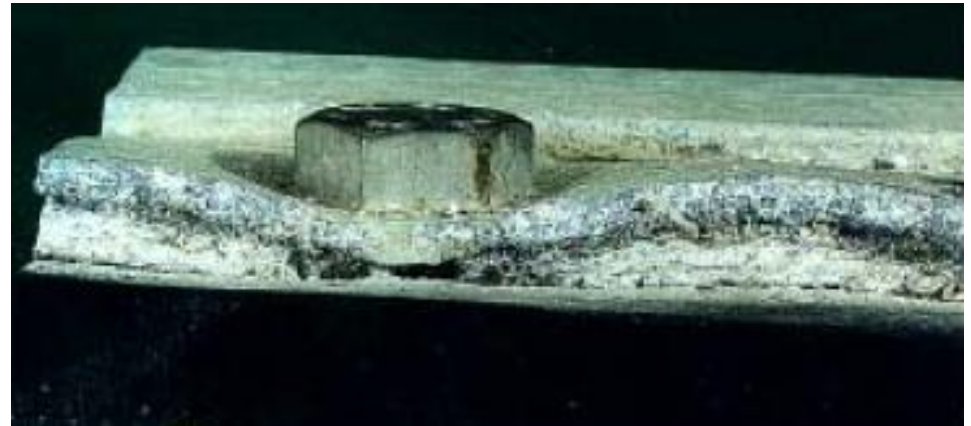
Corrosion of Al in contact with a gasket in graphite containing rubber
